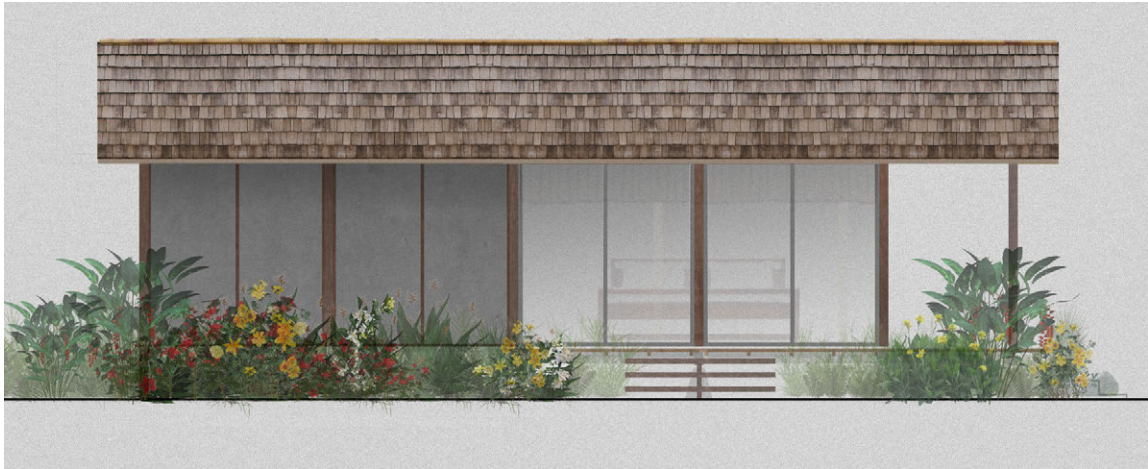
top : Timber Tent with hardwood infill + bamboo shingles roofing bottom : Timber Tent with bison board infill + bamboo shingles roofing
